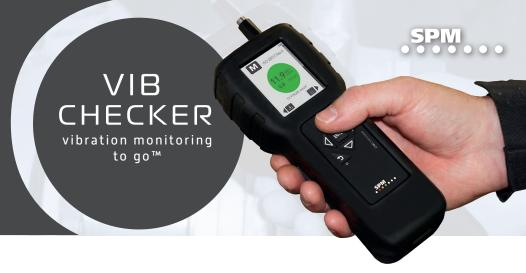
VibChecker is a compact-sized instrument for vibration measurement in the 10-1000 Hz frequency range. Measurement results are immediately and automatically evaluated against ISO standards with a clear, intuitive indication of vibration severity. Time signals and real-time FFT spectrums enable easy pattern recognition. Measurement results can be stored for trending of vibration levels and follow-up.
